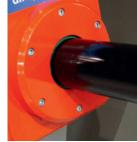
Especially for the Tunnel version: dust cover
