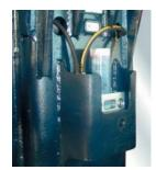
Robust protective housing for the lubricating cartridge
