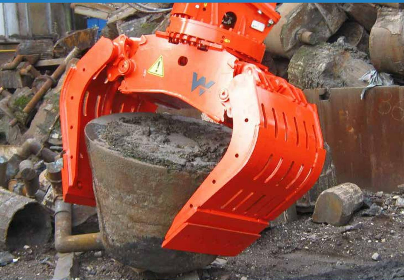
**Grapple** for demolition, sorting and stone positioning
